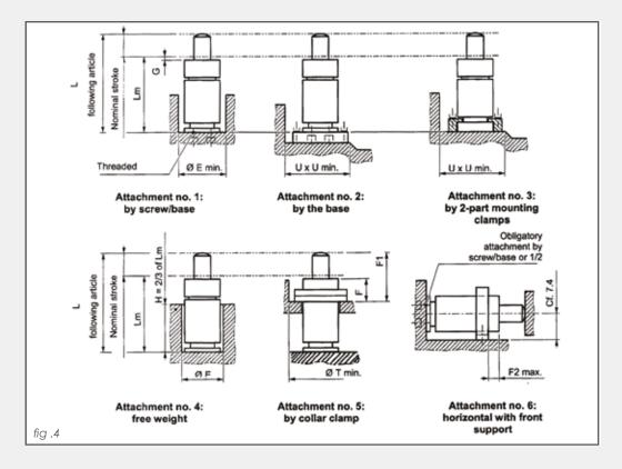
Please note: when method 5 is used the gas spring must always be supported at the base.
